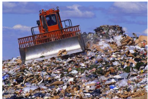
Heavy machinery leveling out landfill waste.
